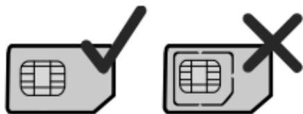
Insert the SIM card in the card slot. Make sure that the SIM card is facing in the right direction, as shown in figure 2, and then slide the SIM card into the slot.
