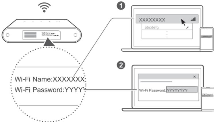
Once the router has connected to a mobile data network, you can connect your computer or mobile phone to the router's Wi-Fi network to access the Internet. Please refer to the label on the bottom of the router for the default Wi-Fi network name (**Wi-Fi Name**) and password (**Wi-Fi Password**).
