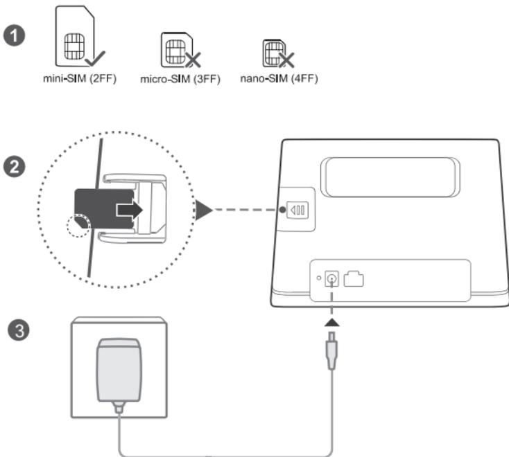
Choose the correct SIM card and insert it into the SIM card slot as shown in the preceding diagram and then connect the power adapter to the router. The router will turn on automatically and search for available mobile networks.
